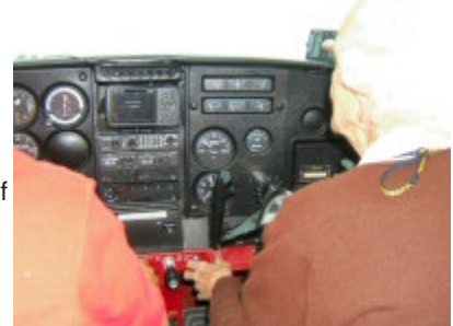
Ruby leans the mixture to achieve peak rpm for the static rpm test.
