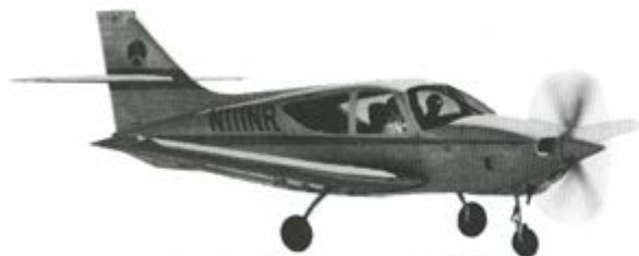
Rockwell Commander 111A*. First all-new, single-engine, fixed-gear plane in a decade.
