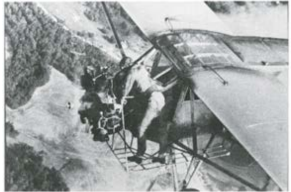
Fred or Al Key on catwalk working on engine. Spark plugs were changed while in flight.
