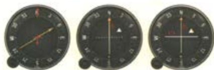
Standard avionics package includes ADF, dual VOR's and glideslope.
